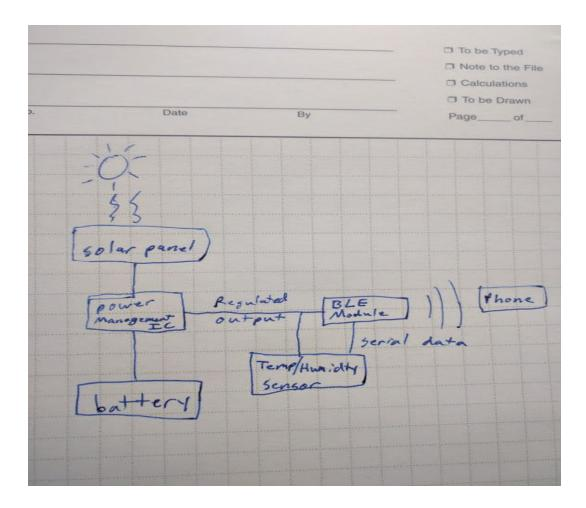
The block diagram shows how to build the circuit system about our project. First of all, temperature and humidity sensor will be connected to BLE module. Secondly, measuring all possible power consumption and get ideal battery for the circuit. Before connecting to the solar panel, transmission task will be done. We decided to use Android application to get data by the transmission. Lastly, get adaptable solar panel and apply it to the circuit.
