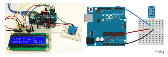
The left picture is the actual circuit which uses screen board. The right picture is a circuit diagram which shows the connection between arduino board and dht11 sensor. This previous project shows us one way to make the temperature circuit. We can see how the circuit will display and how the circuit will be work in the pictures.
