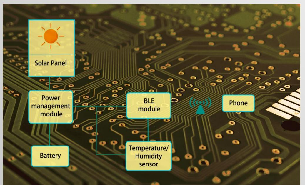
In the system we design to reuse **solar panel** to get solar power.
