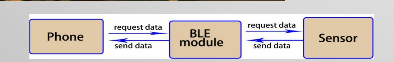
The **BLE module** will generate data from **temperature and humidity sensor** and send it to **mobile devices**.
